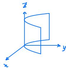
parabolic cylinder along z-axis
